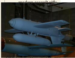
ABOVE - The Henschel Hs 293 was a World War II German anti-ship guided missile: a radio-controlled glide bomb with a rocket engine slung underneath it. It was designed by <u>Herbert A. Wagner.</u>
